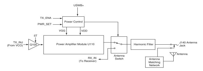
Figure 10-2. UHF Transmitter Block Diagram
