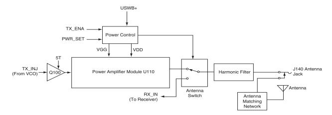
Figure 5-2. VHF Transmitter Block Diagram
