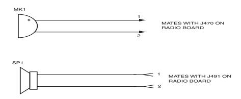
Figure 7-2. Speaker and Microphone Schematic
