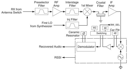
Figure 10-1. UHF Receiver Block Diagram
