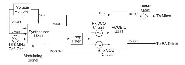
Figure 4-3. VHF Frequency Generation Unit Block Diagram
