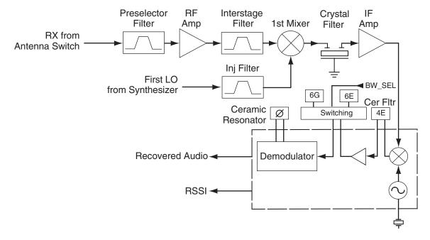
Figure 4-1. VHF Receiver Block Diagram
