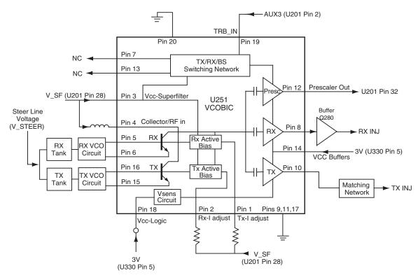
Figure 5-5. VHF VCO Block Diagram
