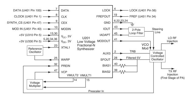
Figure 10-4. UHF Synthesizer Block Diagram
