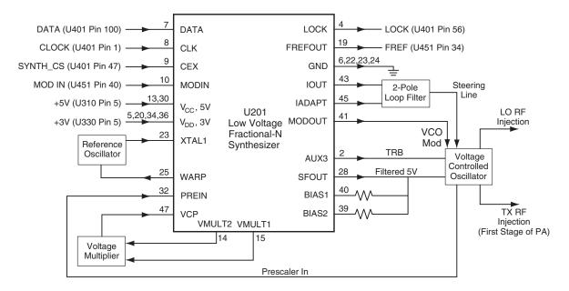
Figure 5-4. VHF Synthesizer Block Diagram
