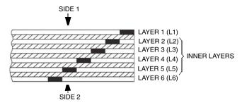
Figure 13-1. Six-Layer Circuit Board: Copper Steps in Layer Sequence
