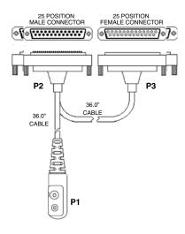
Figure 1-1. Programming/Test Cable
