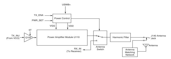
Figure 4-2. VHF Transmitter Block Diagram
