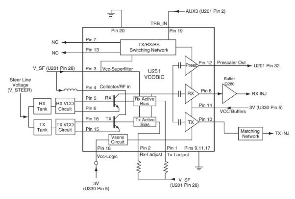
Figure 11-5. UHF VCO Block Diagram
