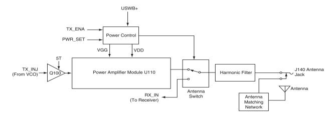
Figure 8-2. UHF Transmitter Block Diagram
