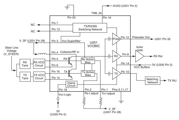
Figure 4-5. VHF VCO Block Diagram
