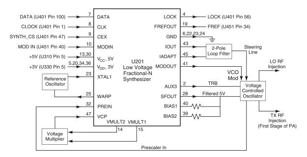
Figure 9-4. UHF Synthesizer Block Diagram
