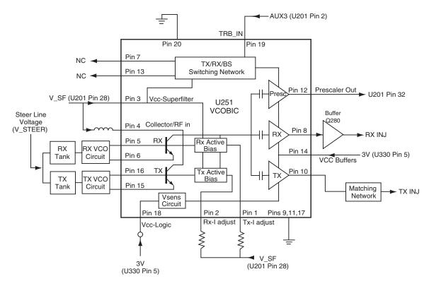
Figure 10-5. UHF VCO Block Diagram
