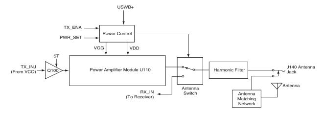
Figure 9-2. UHF Transmitter Block Diagram
