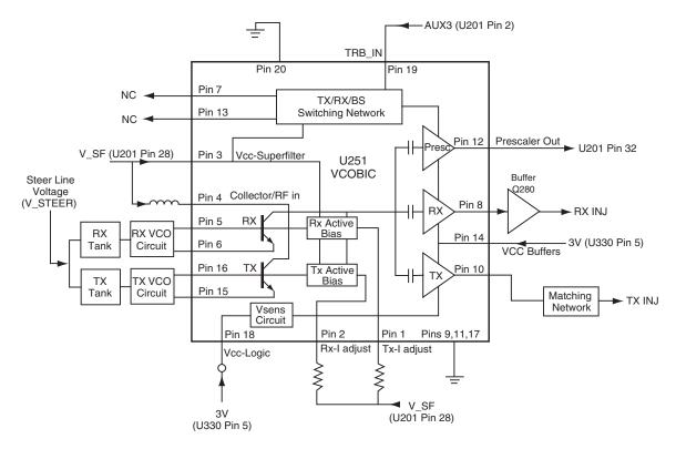
Figure 8-5. UHF VCO Block Diagram
