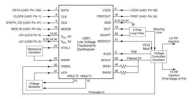
Figure 11-4. UHF Synthesizer Block Diagram
