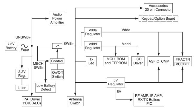
Figure 2-1. DC Power Distribution Block Diagram
