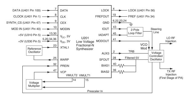
Figure 8-4. UHF Synthesizer Block Diagram
