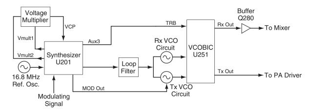
Figure 11-3. UHF Frequency Generation Unit Block Diagram
