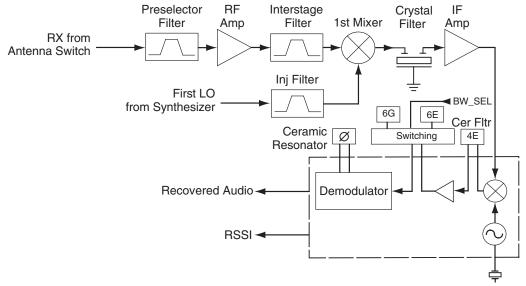
Figure 11-1. UHF Receiver Block Diagram
