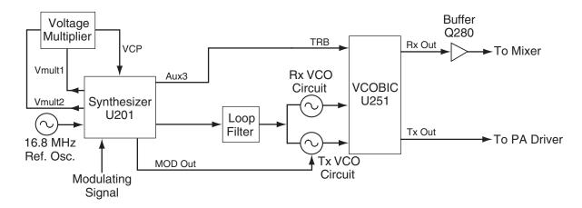
Figure 10-3. UHF Frequency Generation Unit Block Diagram
