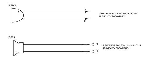
Figure 13-2. Speaker and Microphone Schematic
