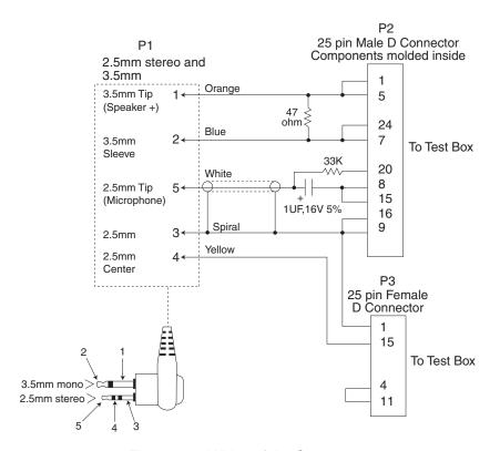
Figure 1-2. Wiring of the Connectors
