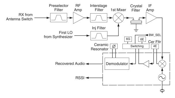
Figure 5-1. VHF Receiver Block Diagram
